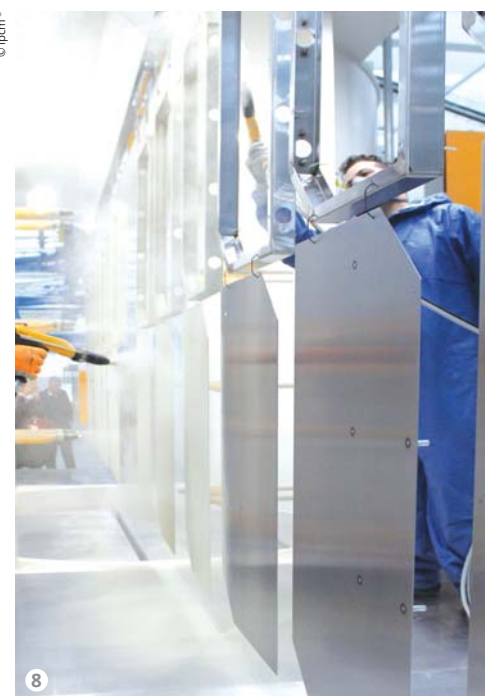
Figure 8: Both booths are equipped with pre and post-retouching stations.
