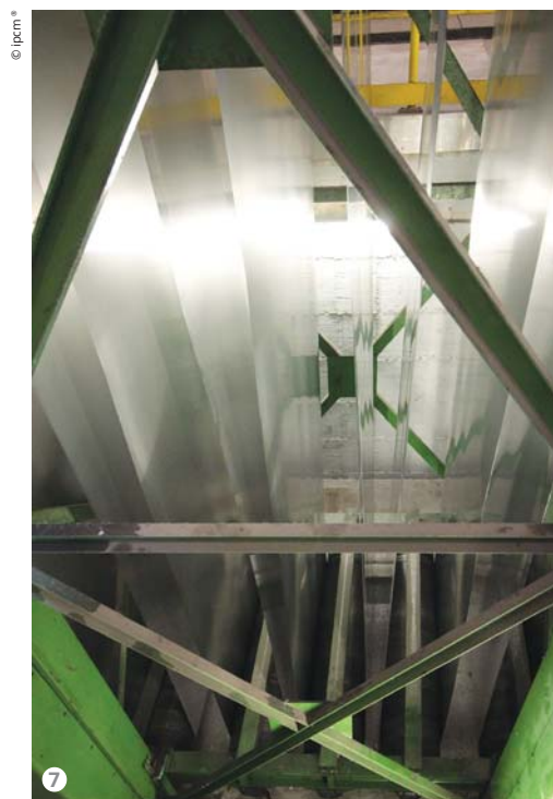
Figure 7: Accumulators at both the entrance and exit allow to continuously coat without ever stopping the system.
