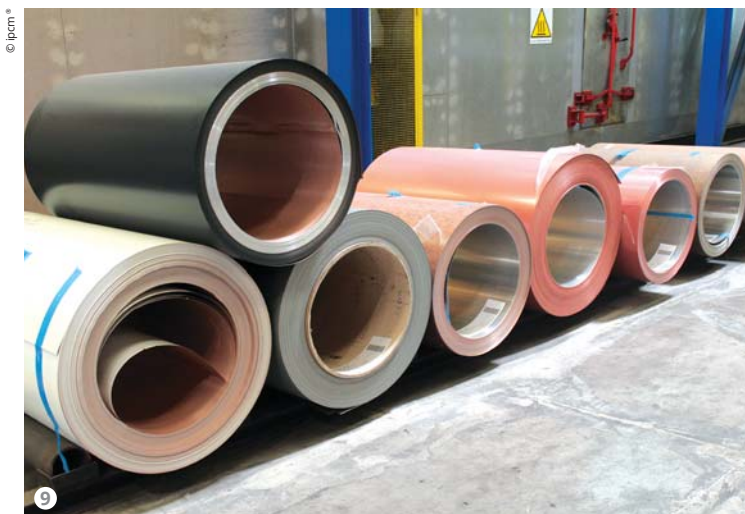
Figure 9: Coils painted with different effects: from the copper-like finish to the oxidised-like and matte ones.
