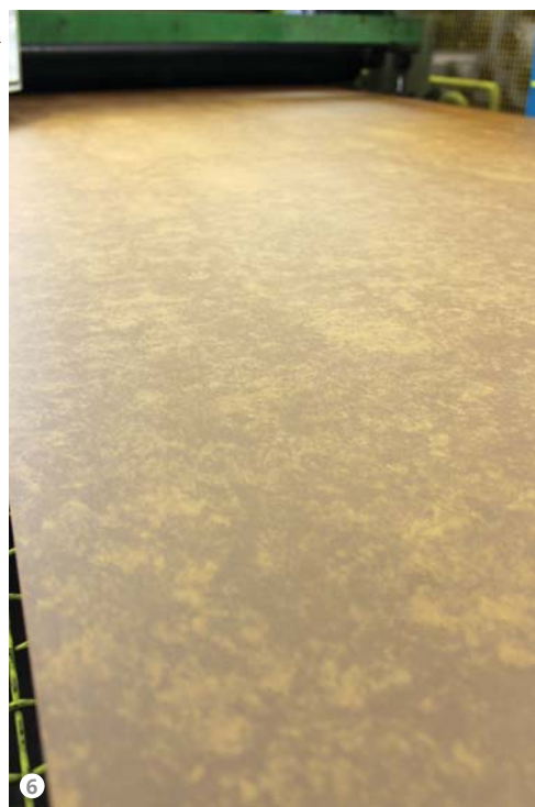
Figure 6: A coated coil exiting the curing oven and passing through the quality control area.
