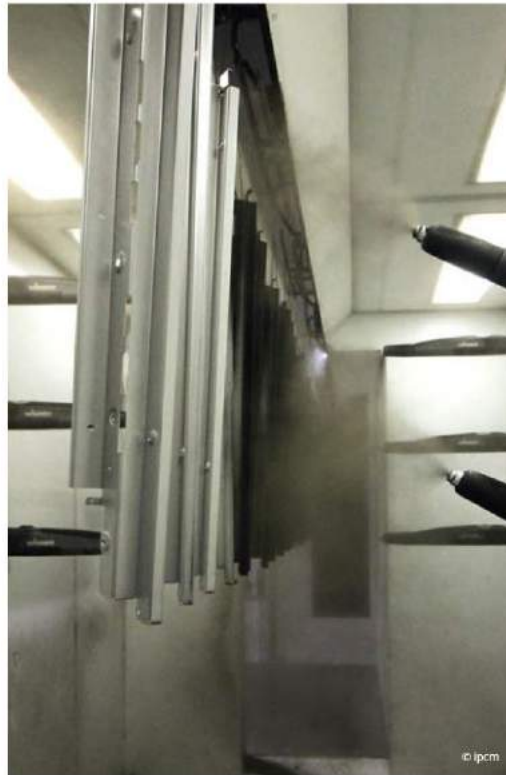
The application of powder coatings.
