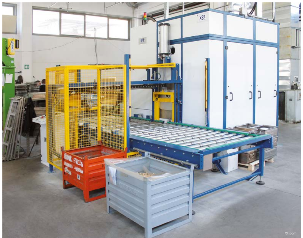
The handling system that takes the baskets carrying the small parts to be treated inside the cleaning machines and the IFP Europe cleaning systems.
